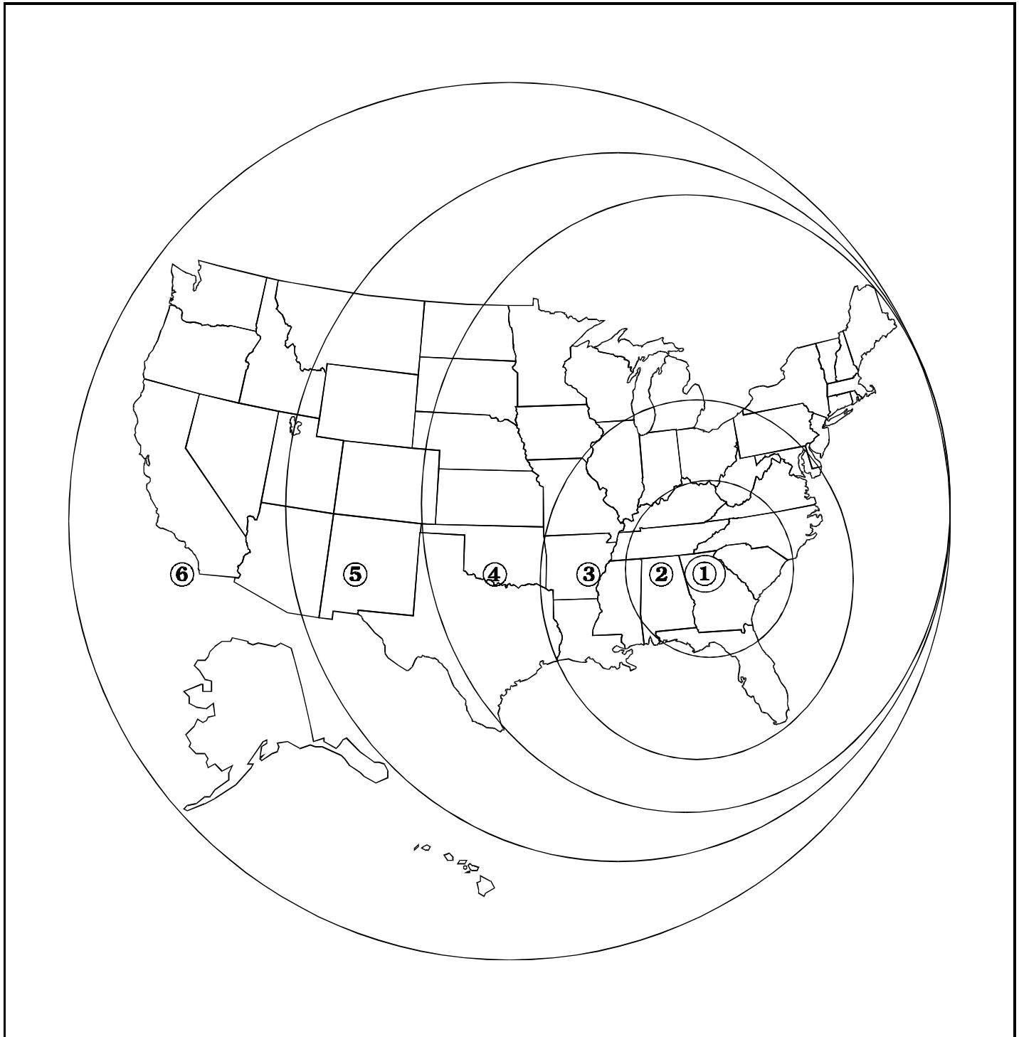
Figure A-10. Example Carrier C Simplified WATS Service Bands for Atlanta
